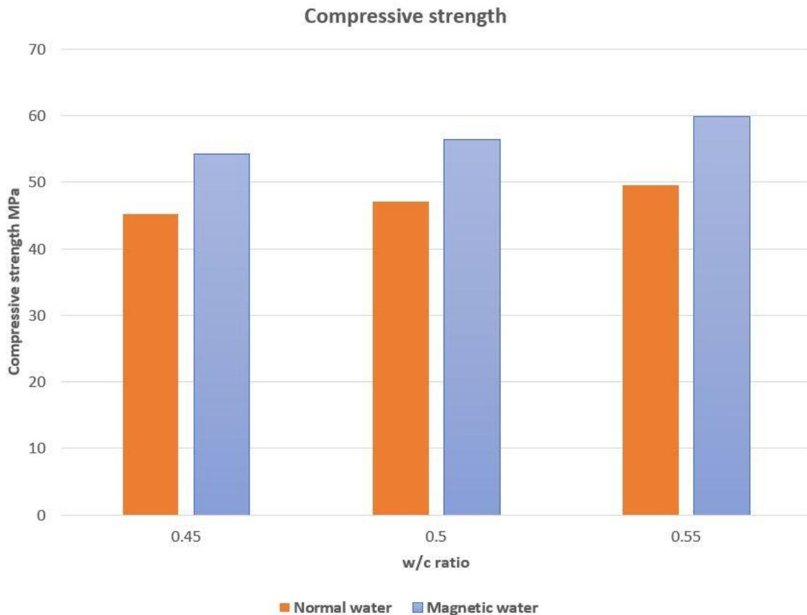
**Figure 5** Variation of compressive strength with w/c ratios
