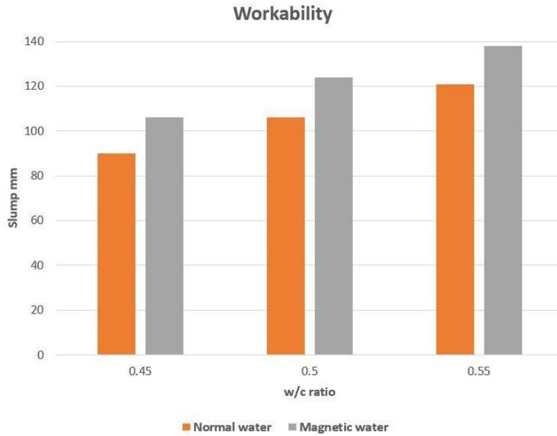
**Figure 3 Variation of slump with w/c ratio**
