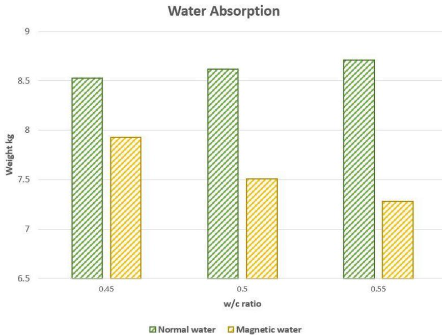
**Figure 4 Variation in weight of concrete with different w/c ratio**
